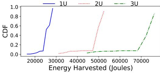
Fig. 2: Impact of satellite size on energy harvested
