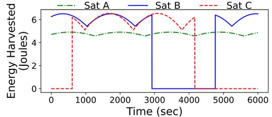
Fig. 1: Energy Generated by 3 satellites over 100 minutes
