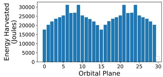
Fig. 4: Impact of orbital plane position on energy harvested with satellites at 400 km altitude with an inclination angle of  $95^\circ$  to observe the impact of the orbital plane position (Fig 4). The position of the orbital plane will determine how long a satellite will be in eclipse, as well as the incidence angle of sun light. Both these factors contribute to the observed variations.
